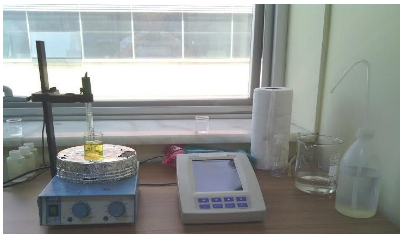
Fig. 2: System of potentiometric titration cell used in studied
