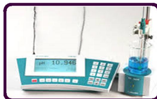
Fig. 2: System of potentiometric titration cell used in studied
